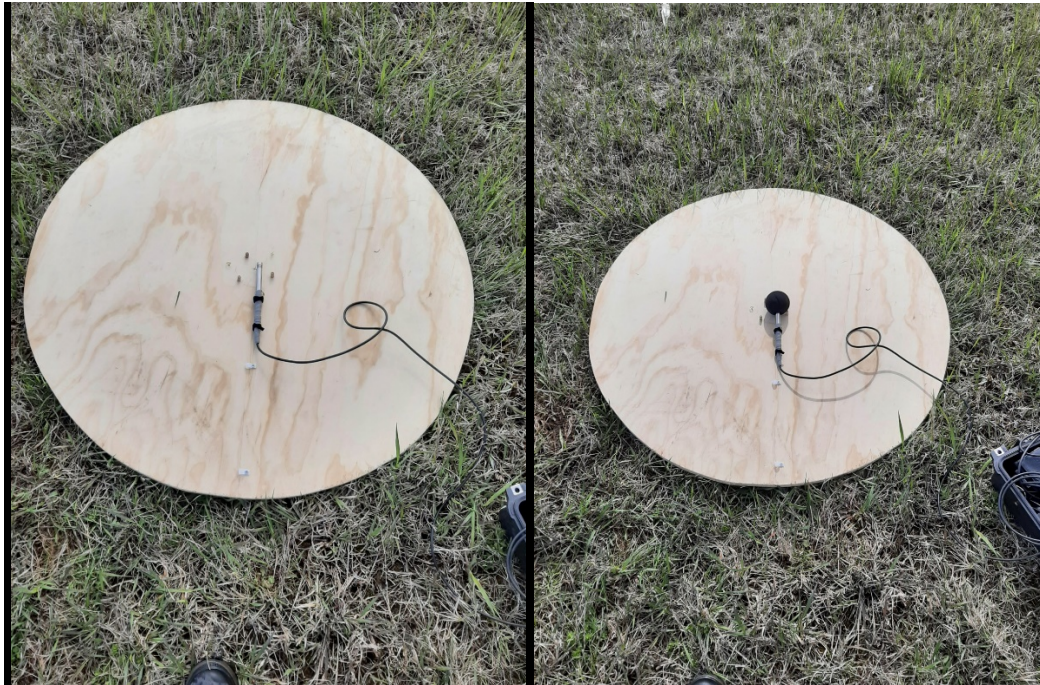
Sound Level Microphone on Board, Upwind – April 22, 2021
