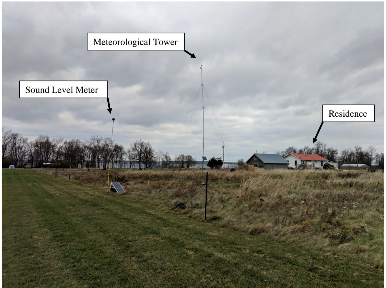
Photo of Meteorological Tower and Sound Level Meter at Location M316 (looking north)
