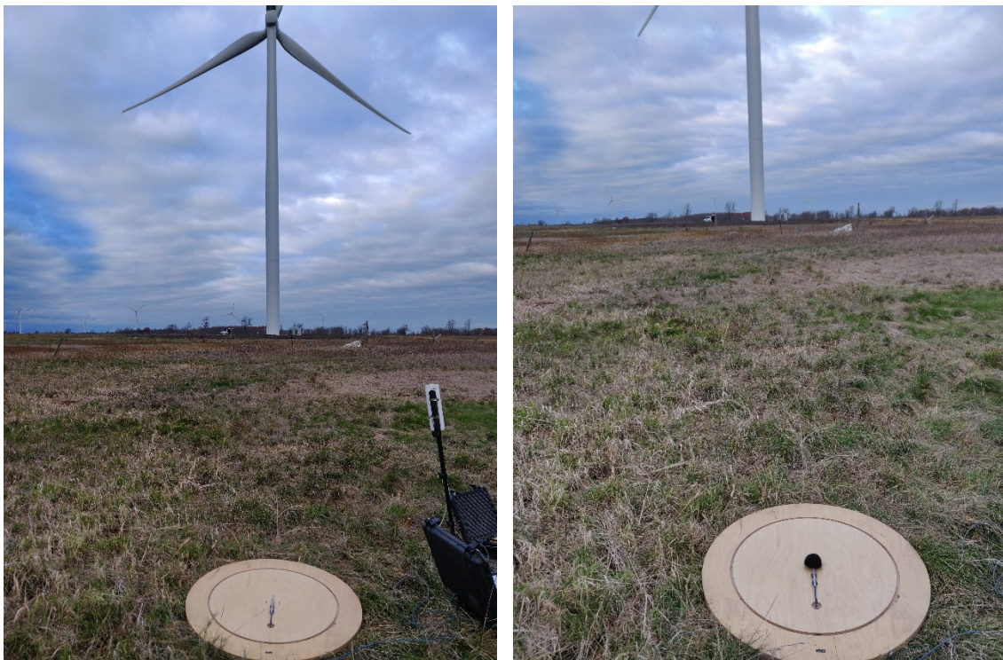
Sound Level Microphone on Board - November 8, 2018
