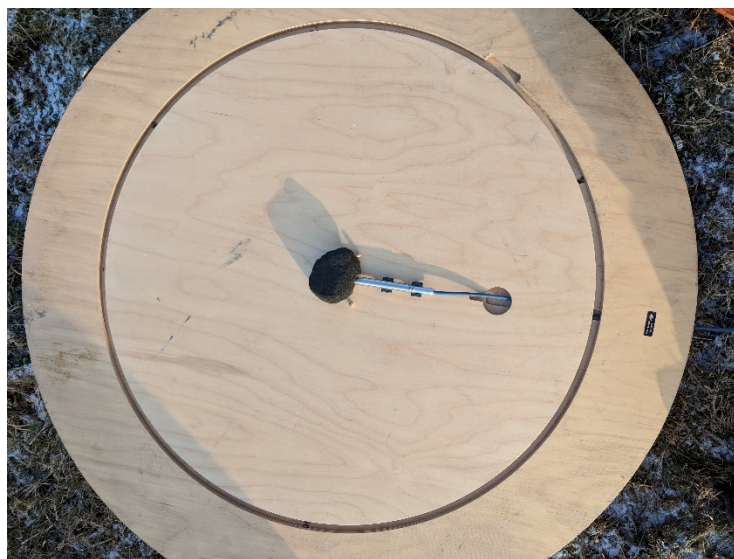
Sound Level Microphone on Board - December 6, 2018
