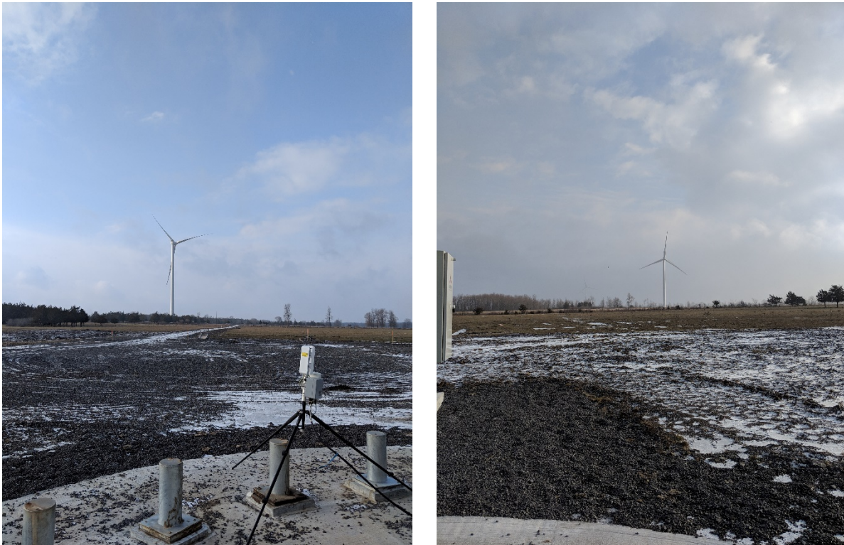
Photos of Sound Level Meter and Meteorological Tower Taken from the Base of WTG S29
